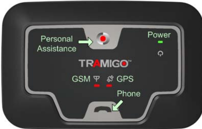
Figure 4 - T22 Control Panel
