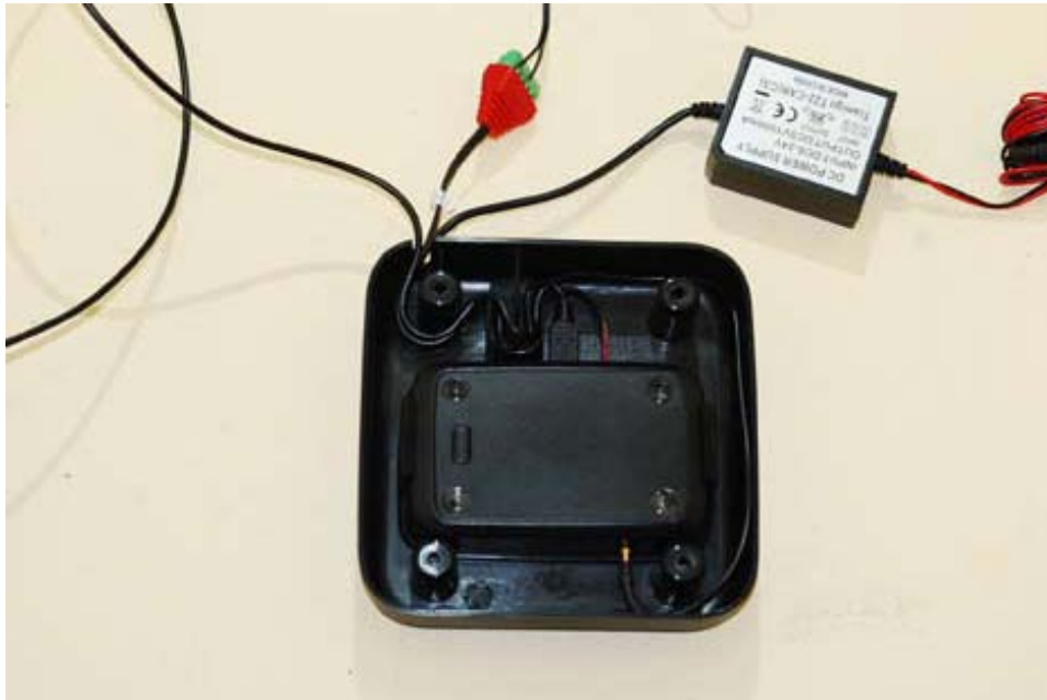
Figure 3 - T22 Automotive Installation Case
