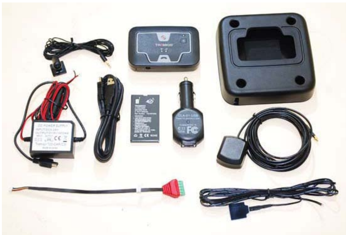
Figure 1 - T22 and Automotive Installation Kit
