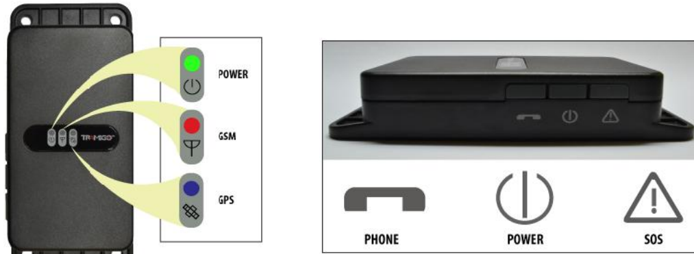
Figure 1 – T23 and T23 Fleet Unit Controls
